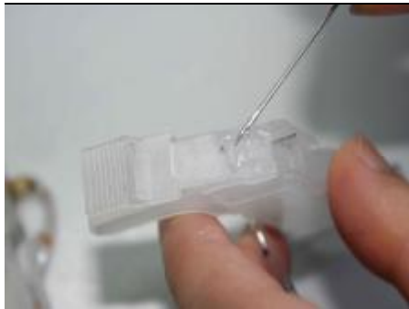
Put glue at the same position of the refilling cartridge (at the 2 sides)
