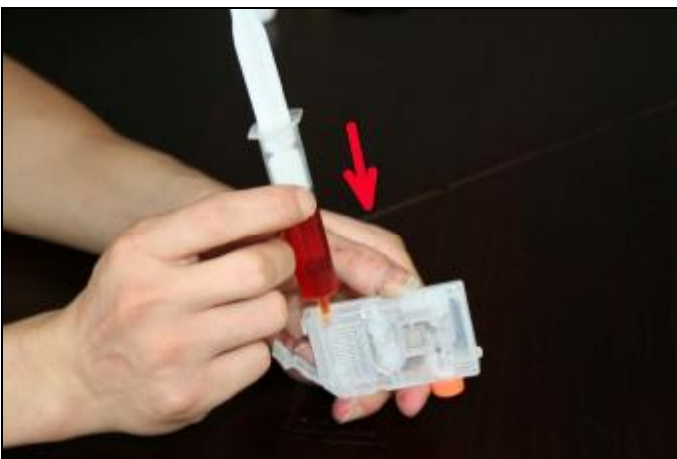
Use the syringe to draw some ink, and then insert the syringe into the cartridge
