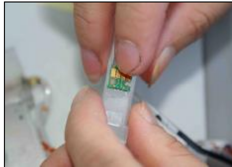
Stick the chips on the refilling cart (Pls note that the color should be correct. Do not mix the chips)
