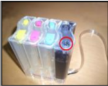
Insert the syringe in the ink filling hole, Then, cover air hole Fill 2/3 ink into the reservoir bottle
