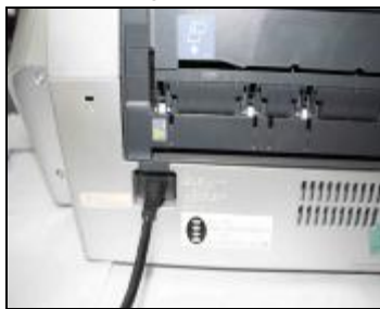
Insert the electrical source line suitably
