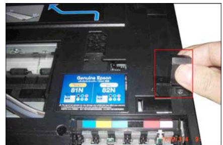
Place the black position-limit part as above picture shown
