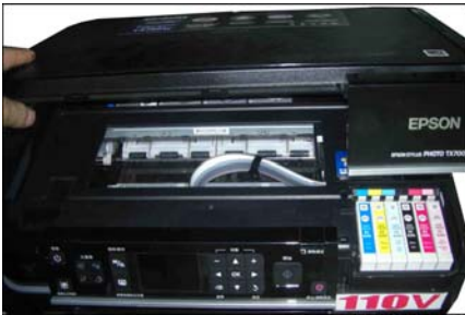
Open the printer cover
