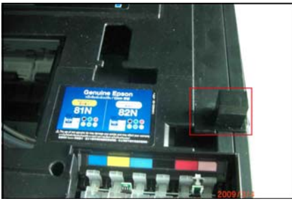
Position-limit part well installed
