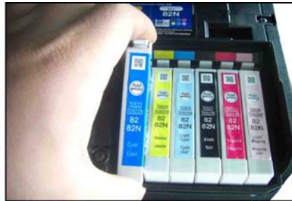
take out the original cartridges
