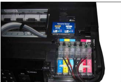
Place CIS cartridges into the carriage
