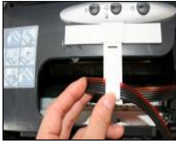
Insert tubeline through the arm
