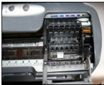
Remove original cartridge
