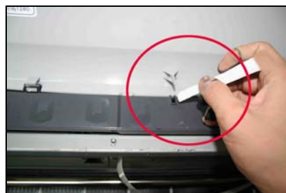
During printing, pls keep the Cover of the printer open, just insert the paper to the hole as picture shows. Then no need to close the cover.
