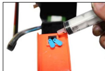
Put the inkjector to the hole that you are going to draw air out
