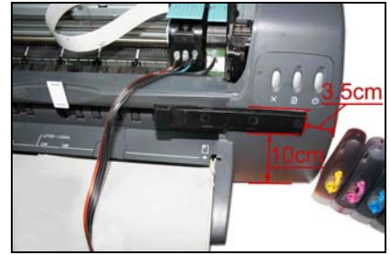
Put the long support arm 3.5cm right to the short one and 10cm down.
