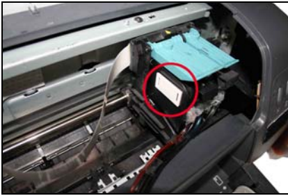
We have installed the support arm in the cartridges
