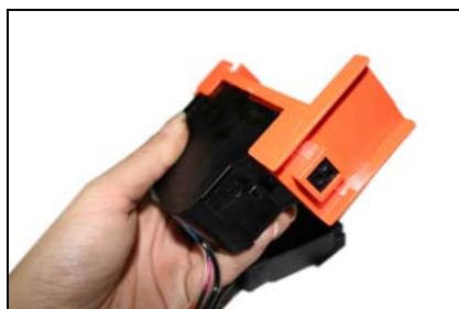
Put out the cartridges and put in the pedestal, install it on the end with hole
