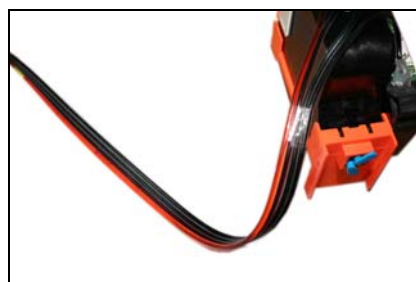
In the same way, draw out the air for other color cartridges, then there will be no air in the tubes.
