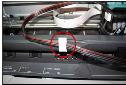
Close the tubes to the support arm by clasp, and make sure the tubes are not contorted
