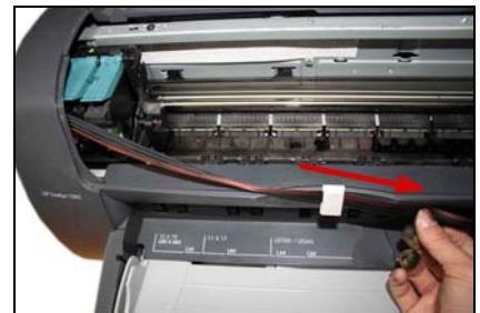
pull the tubes straight, the tube can not be that long or contorted.
